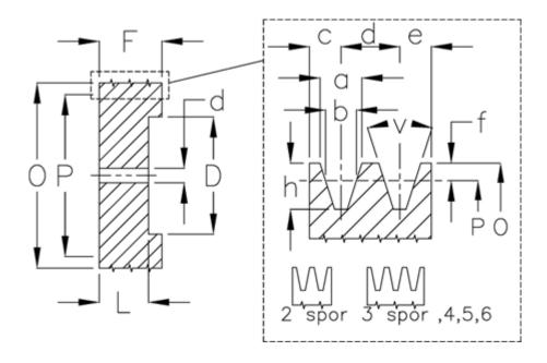
$\begin{array}{lll} D & = 67 \\ d & = 15 \\ F & = 65.0 \\ L & = 52 \\ Number of ribs = 4 \\ O & = 105.5 \\ P & = 100 \\ Type & = A \end{array}$
